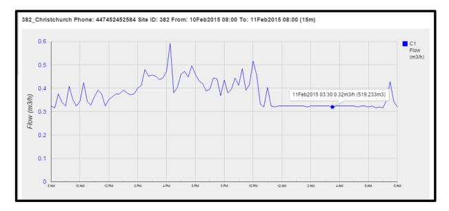
Snapshot of water data logger over last 24 hours. You can see the varying flow rate whilst the site is in use throughout the day and once the site closes at approx. 10.30 pm, there is no variation in flow rate as nothing is being turned on and off, but there is a constant flow of water running throughout the night from a source of approx. 0.32m<sup>3</sup> per hour.
