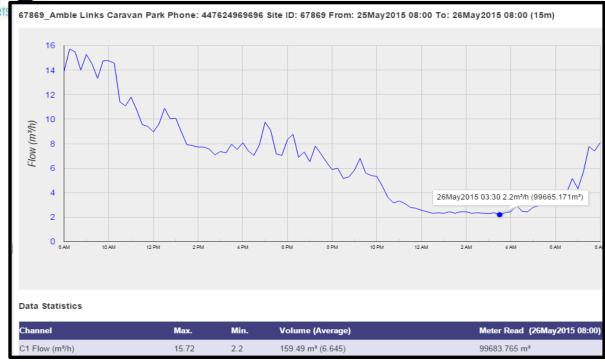
Snapshot of water data logger monitoring water meter 10XH12345 as at 03.30am this morning, Tuesday 26<sup>th</sup> May, where a minimum flow rate of 2.2m³ per hour (2,200 litres) was being recorded.
