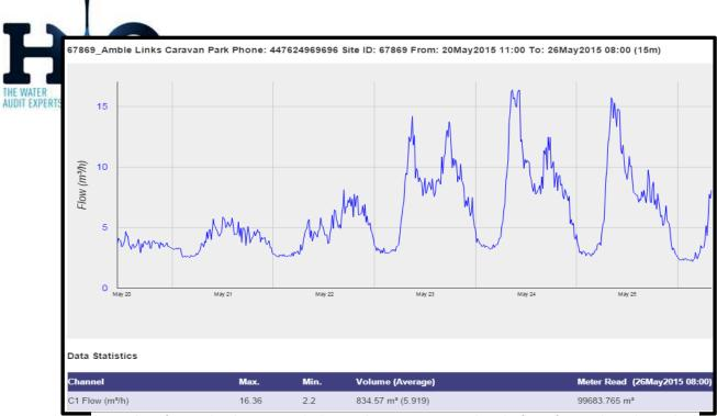
Snapshot of water data logger over the last week. As you can see, when the flow of water drops during the middle of the night when nobody is using water on park, there is still a constant flow of water running through the meter which never drops below 2.2m³ per hour
