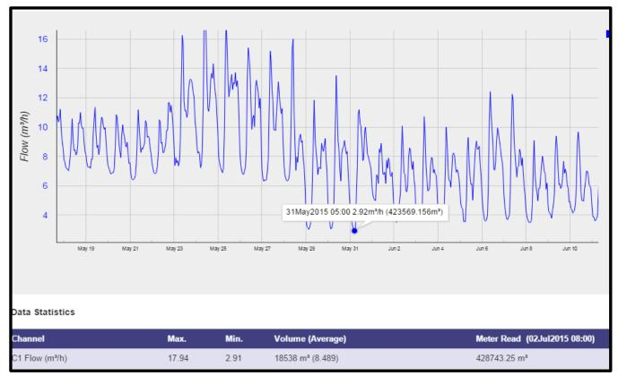
Now water leak repairs have been completed, the minimum overnight flow rate has dropped to an average of 3m<sup>3</sup> per hour.
