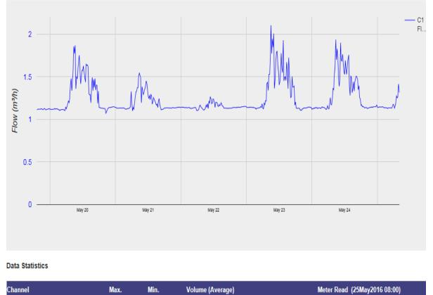
Snapshot of water data logger between the hours of 00:00am-06.00am reflecting an overnight flow rate of at least 1.14m<sup>3</sup> per hour
