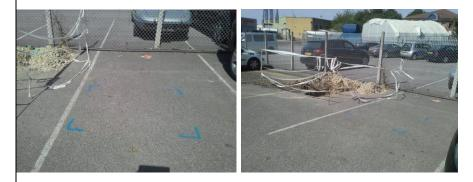
The best source of surface noise was marked with the centre position being 2.1m from the existing excavation and 2.7m from the boundary fence.
